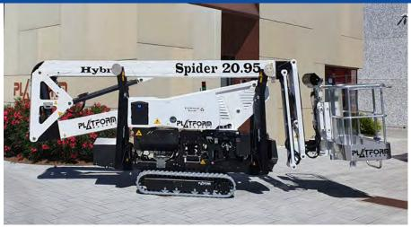
The newly released 2095 is the best performing Spider Lift that weighs under 3.5 t including a trailer. This means that this machine could be towed behind most tradesmen's vehicles.
