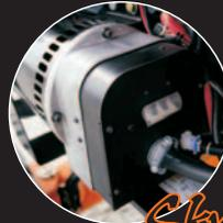
JLG delivers more power where you need it with the SkyPower™ Package. Machines outfitted with the SkyPower Package include a 7500W self-contained generator, plus a power cable and a 1/2 inch air line routed through the boom's power track to the platform. As an added benefit, the SkyPower Package is designed to work with various add-on accessories, including the SkyWelder™ Package.
